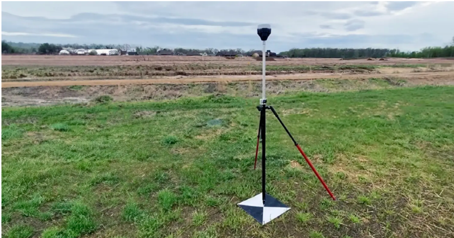
Above: Typical GNSS receiver setup for drone work with ground control point (GCP) marker. photo by: https://emlid.com/drone-mapping/
